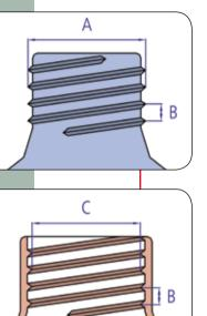
Plastic barrels and containers can have a wide range of thread types. Some are standardized according to DIN, BSI or US standards. Other threads are manufacturer-specific. We can supply suitable adapters for most containers so that discharge valves, pumps and other accessories can be safely attached.
